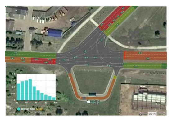
Figure 2 – The results of the test of the intersection model with the current parameters of the traffic lights
