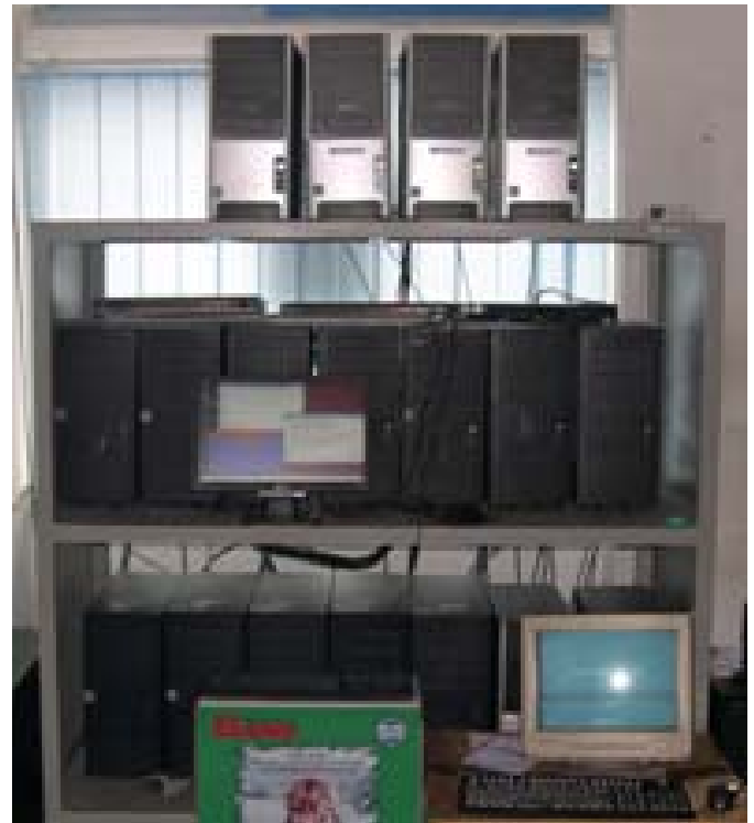
Fig. 1 PC cluster built at the National Institute of Aeronautics and Space (LAPAN), Bandung.
