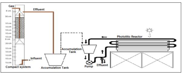
Fig. 1 Schematic of anaerobic reactor followed by Solar Photocatalitic Reactor
