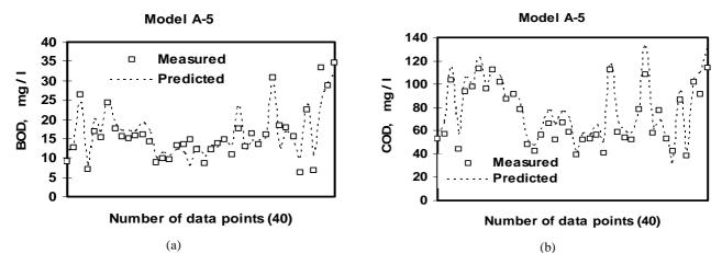
Fig. 6 Measured and predicted test data for (a) BOD and (b) COD concentration from Model A-5.
