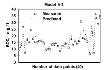
Fig. 4 Measured and predicted test data for BOD concentration from Model A-3.
