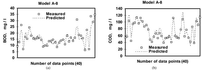
Fig. 9 Measured and predicted test data for (a) BOD and (b) COD concentration from Model A-8.
