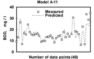
Fig. 12 Measured and predicted test data for BOD concentration from Model A-11.
