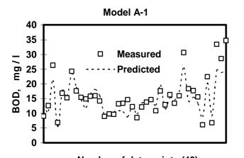
Number of data points (40) Fig. 2 Measured and predicted test data for BOD concentration from Model A-1.
