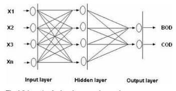
Fig. 1 Schematic of a three layer neural network.
