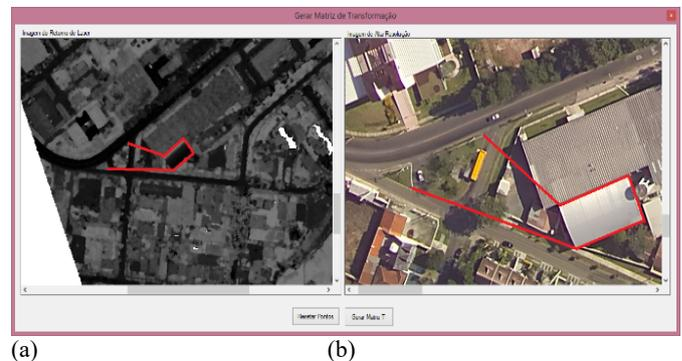
Fig. 5 Selection of common points between the image generated from the laser data (a) and the high resolution image (b) to perform matching.
