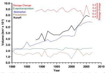
**Fig. 4** Plot of the hydrological parameters used in the estimation of runoff in the Reservoir.
