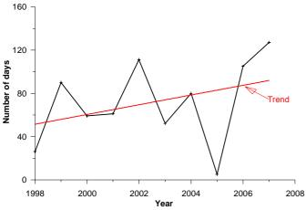
**Fig. 5** Plot of number of days spillgate has been opened from 1998 to 2007 and a trend on the data.
