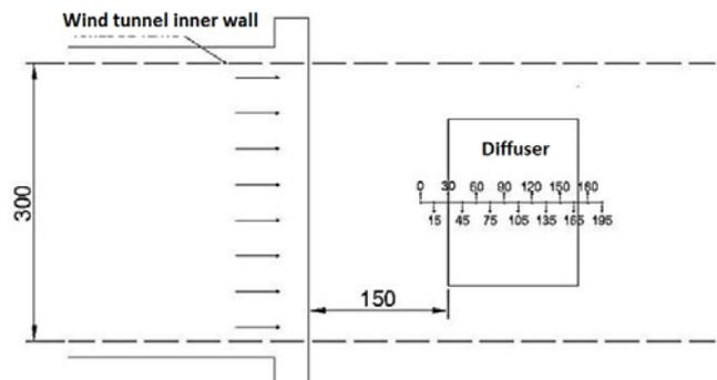
**Fig. 2** Distance between the diffuser and the wind tunnel exit.
