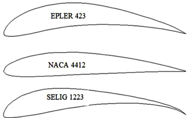
Fig. 5 Airfoils used in the diffusers.
