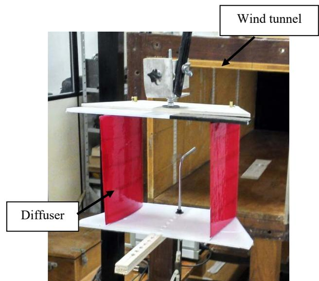
Fig. 6 Diffuser positioned at the wind tunnel exit.
