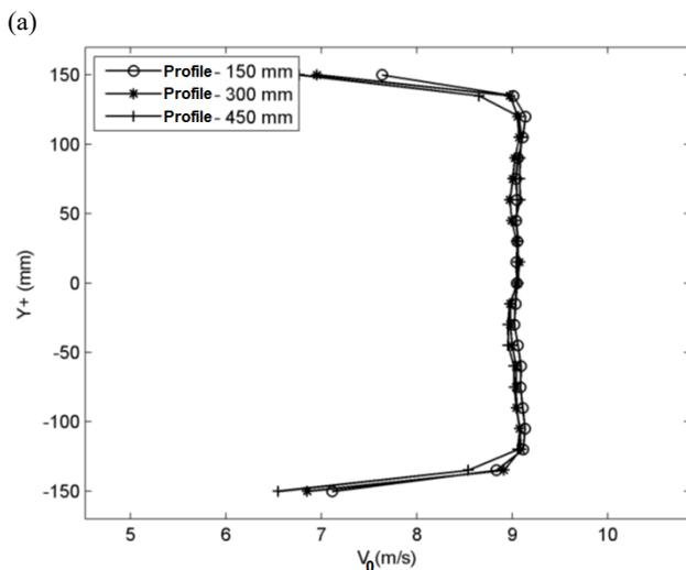
**Fig. 7** Wind profile outside the wind tunnel in the three points measured for (a)  $V_0 = 4\text{ m/s}$  and (b)  $V_0 = 9\text{ m/s}$ .
