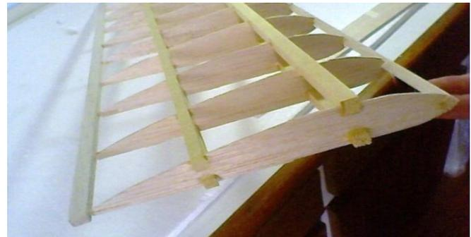
**Fig. 1** Design of the airfoil and alignment for assembling the diffuser.
