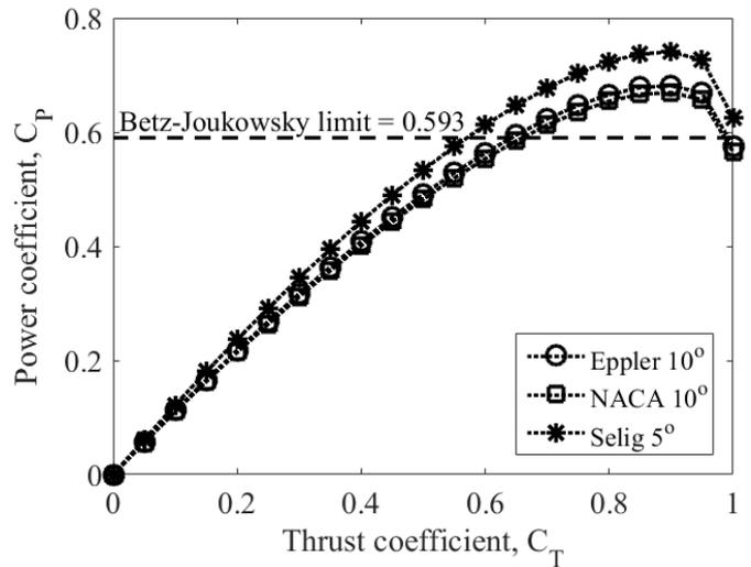
**Fig. 9** Power coefficient as a function of the thrust coefficient.
