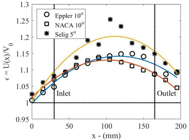
**Fig. 8** Comparing the velocity ratio results of the diffusers for  $V_0 = 6\text{m/s}$ .
