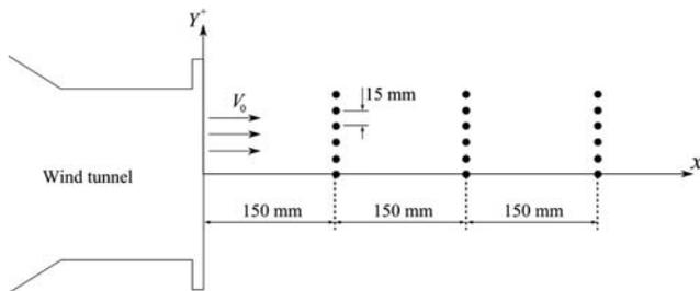
Fig. 3 Measuring points for the velocity profiles outside wind tunnel.
