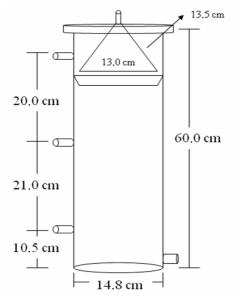
Fig. 2 (a) Schematic representation of UASB reactor.
