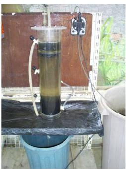
Fig. 2 (b) Picture of the Upflow Anaerobic Sludge Blanket (UASB).
