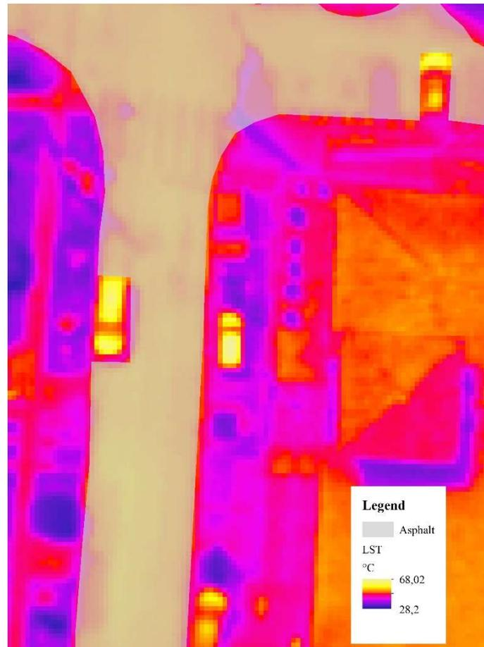
Fig. 5 Thermal image of the same locality shown in 0 and segmented area for asphalt analysis.
