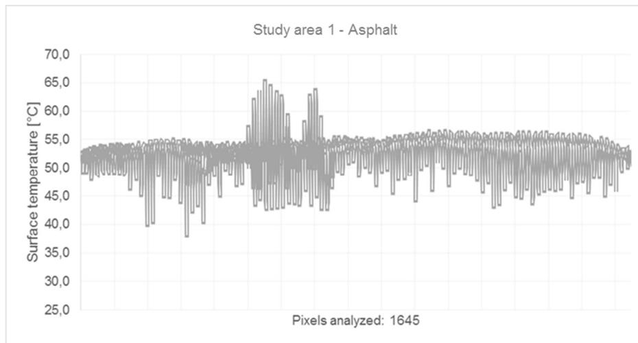
**Fig. 7** Distribution of surface temperature of asphalt in study area 1.
