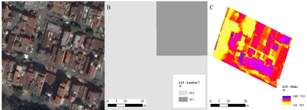
**Fig. 3** Comparison between LST values derived from Landsat 7 (B) and the thermal sensor used in this study (C).
