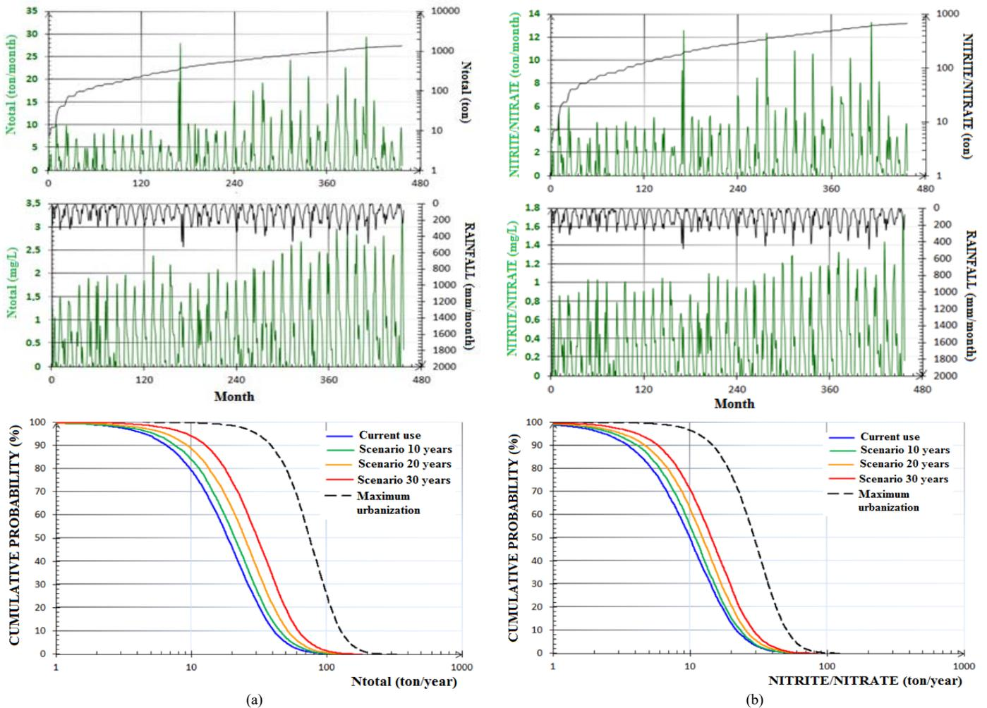
**Fig. 6** Series of probable loads and concentrations in Lageado Basin, considering a 38-year horizon for: (a)  $N_{total}$  and (b) nitrite and nitrate.
