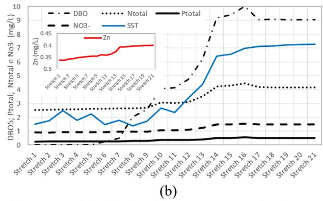
**Fig. 4** (a) Identification of stretches 9 and 16 of Lageado Stream; (b) Longitudinal distribution of the concentrations of pollutants in Lageado Stream for the 30-year urbanization scenario.
