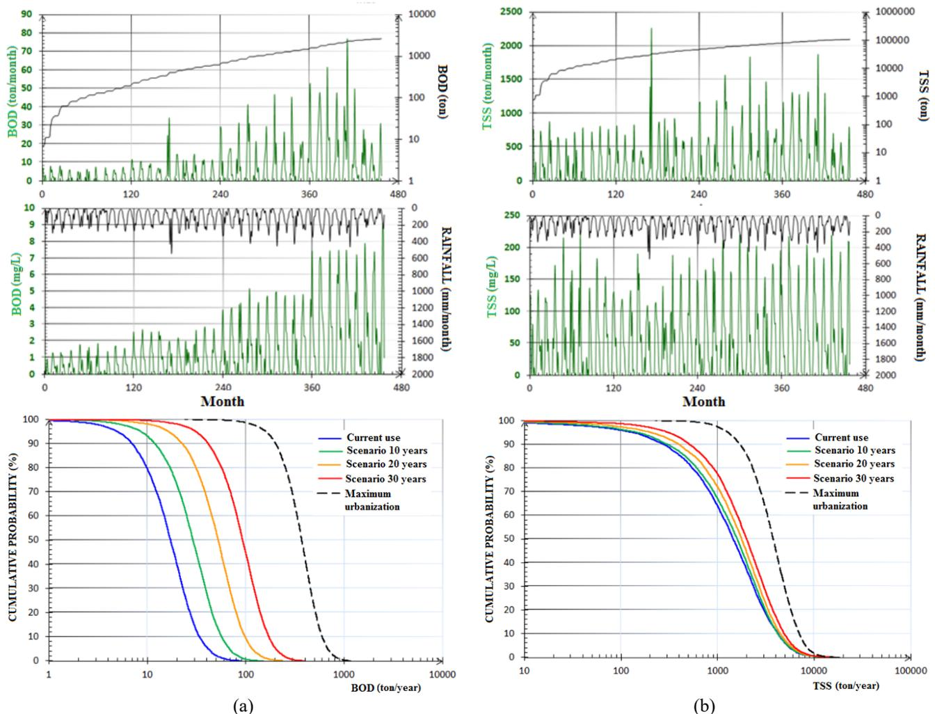
Fig. 5 Probable series of loads and concentrations at the outlet of Lageado Basin, considering a 38-year horizon for: (a) BOD; and (b) TSS.
