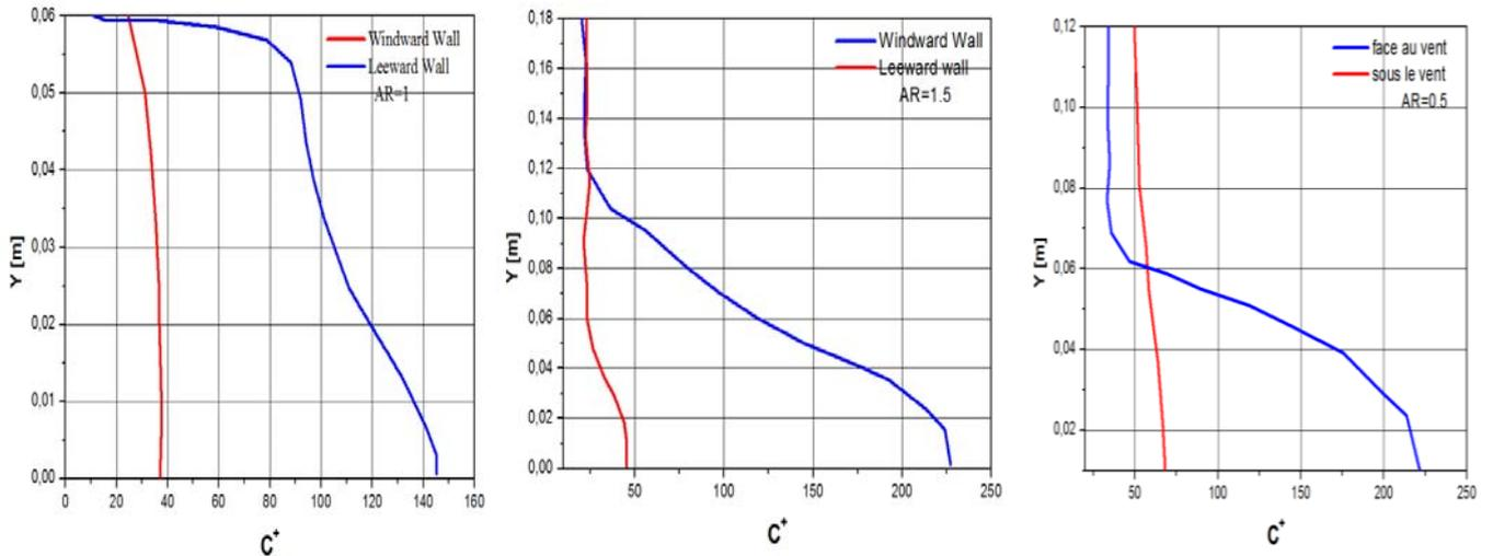
**Fig.7** Dimensionless pollutant concentration  $C^*$ , on the windward wall and the leeward wall for the model with two adjacent boundary walls,  $H_1/H_2=1; 0.5; 1.5$ .
