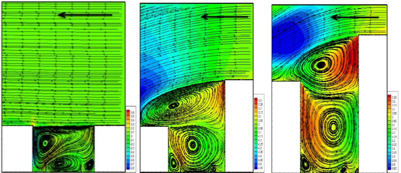
**Fig.5** Contour of vertical Velocity and distribution of the vertical velocity inside the street canyon for the model with two adjacent boundary walls  $H_1/H_2=1; 0.5; 1.5$ .
