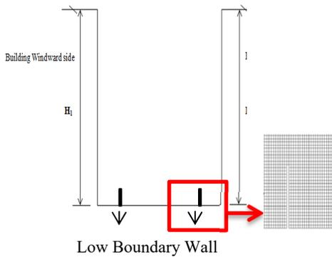
**Fig.2** (a) Street canyon model with two adjacent boundary walls (b) Grid used in CFD simulations for local case.
