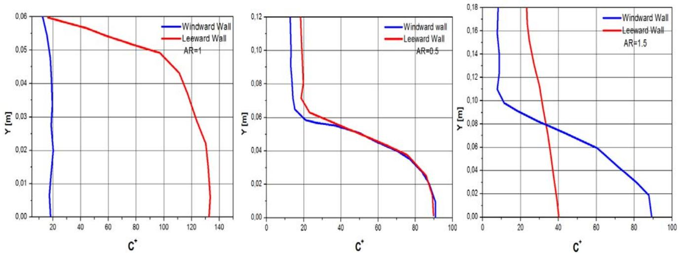
**Fig.8** Dimensionless pollutant concentration  $C^*$ , on the windward wall and the leeward wall for the model with two adjacent boundary walls,  $H_1/H_2=1; 0.5; 1.5$ .
