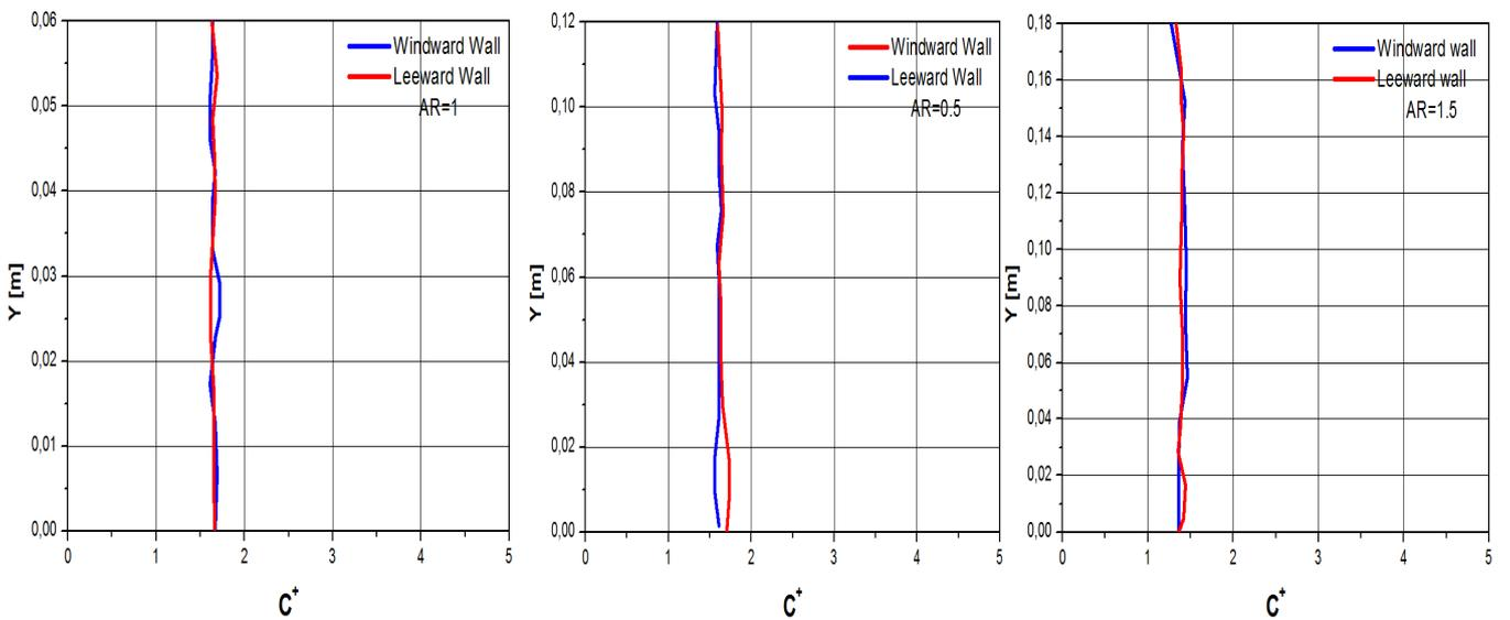
**Fig.9** Dimensionless pollutant concentration  $C^*$ , on the windward wall and the leeward wall for the model with crossing under building,  $H_1/H_2=1; 0.5; 1.5$ .
