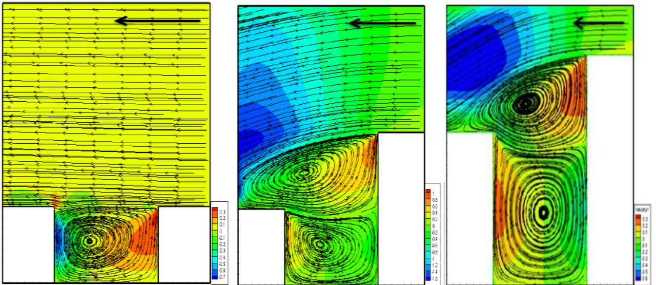
**Fig.4** Contour of vertical Velocity and distribution of the vertical velocity inside the street canyon for the model flat roof-shaped (reference model)  $H_1/H_2=1; 0.5; 1.5$ .
