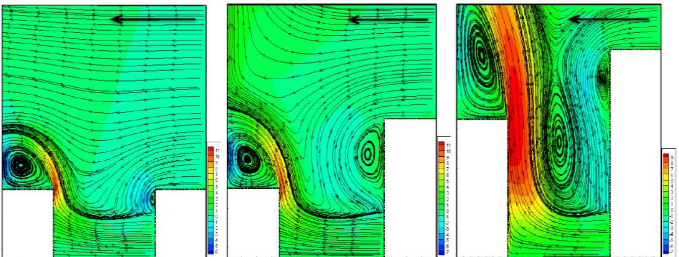
**Fig.6** Contour of vertical Velocity and distribution of the vertical velocity inside the street canyon for the model with Crossing under building  $H_1/H_2=1; 0.5; 1.5$ .
