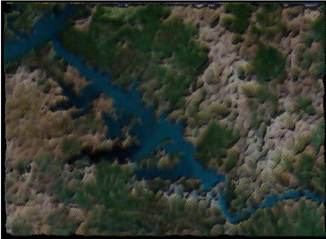
Fig. 9 Digital terrain model of the dataset1 using radial basis and spacing of two by two.
