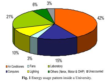
the campus which is also the potential source of CFC emission, which is to be controlled to make the campus a Green campus. The usage pattern is given in **Fig. 1**.
