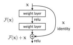
**Fig. 4** Example of a ResNet architecture residual block containing two convolution layers (weight layer) and one activation layer (ReLU) (He *et al.*, 2016).
