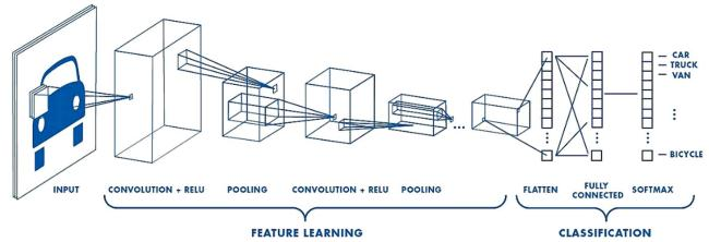
Fig. 3 Illustration of an example of CNN architecture, adapted from Prabhu (2018).
