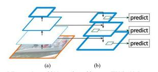
**Fig. 5** Feature Pyramid Network Architecture (FPN). (a) Bottom-up path. (b) Top-down path (Lin *et al.*, 2017).
