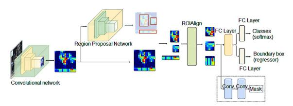
Fig. 2 Network architectures: (a) Faster R-CNN; (b) Mask R-CNN. Adapted from Hui (2018b).
