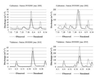
Fig. 3 Simulated and observed streamflows in two rain seasons selected.
