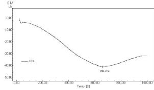
Fig. 5 DTA curve from the differential thermal analysis of the slurry sample.
