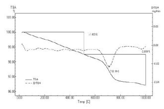
Fig. 4 TG and drTG curves from thermogravimetric analysis of the slurry sample.
