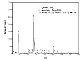
Fig. 3 Result of the XRD analysis of the slurry sample with the peaks indicated and related to the corresponding mineralogy.
