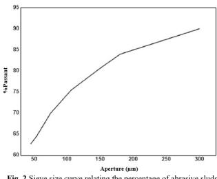
Fig. 2 Sieve size curve relating the percentage of abrasive sludge passing the sieve opening in μm.
