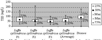
**Fig. 10** Box-whisker graphics for total suspended solids (TSS) downstream the filters filled with *Luffa cyllindrica* (F1, F2, F3 and average value) and downstream the filter filled with stones (upstream the secondary settlers).
