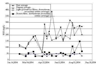
**Fig. 5** Biochemical oxygen demand (BOD5,20) in raw and primary sewage, downstream the trickling filters filled with Luffa cyllindrica and downstream the filter filled with stones: temporal series.
