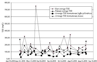
**Fig. 9** Total suspended solids (TSS) in raw and primary sewage, downstream the filters filled with *Luffa cyllindrica* and downstream the filter filled with stones (upstream the secondary settlers): temporal series.
