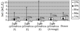
**Fig.12** Box-whisker graphics for settleable solids (SetS) downstream the filters filled with *Luffa cyllindrica* (F1, F2, F3 and average value) and downstream the filter filled with stones (upstream the secondary settlers).
