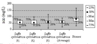
**Fig. 6** Box-whisker graphics for biochemical oxygen demand (BOD5,20) downstream the filters filled with Luffa cyllindrica (F1, F2, F3 and average value) and downstream the filter filled with stones (upstream the secondary settlers).
