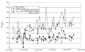
Fig. 7 Chemical oxygen demand (COD) in raw and primary sewage, downstream the filters filled with *Luffa cyllindrica* and downstream the filter filled with stones: temporal series.
