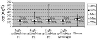
**Fig. 8** Box-whisker graphics for chemical oxygen demand (COD) downstream the filters filled with *Luffa cyllindrica* (F1, F2, F3 and average value) and downstream the filter filled with stones (upstream the secondary settlers).
