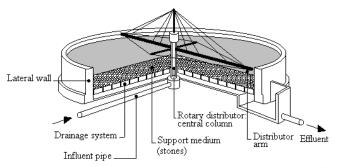
Fig. 1 Typical configuration and main parts of a classic trickling filter. Figure adapted from Jordão and Pessoa (2009).
