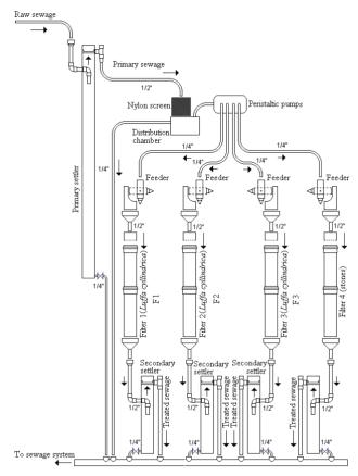
**Fig. 3** General arrangement of the pilot plant, consisting of a primary settler, and four parallel and identical secondary biologic systems, three of them operating with *Luffa cyllindrica* as biofilm support medium (F1, F2, F3), and the last one using stones (filter 4).
