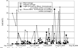
**Fig. 11** Settleable solids (SetS) in raw and primary sewage, downstream the trickling filters filled with *Luffa cyllindrica* and downstream the filter filled with stones: temporal series.
