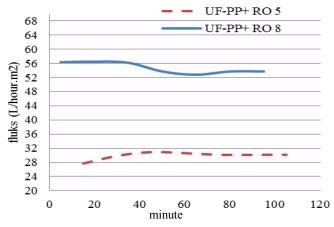
Fig. 8 Flux of RO membrane with UF-PP pretreatment.
