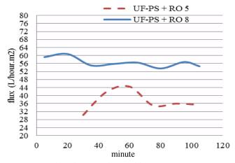
Fig. 7 Flux of RO membrane with UF-PS pretreatment.
