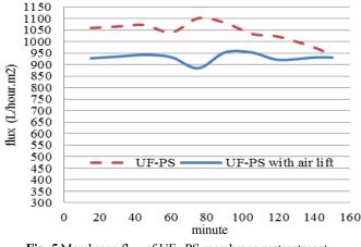
Fig. 5 Membrane flux of UF-PS membrane pretreatment.
