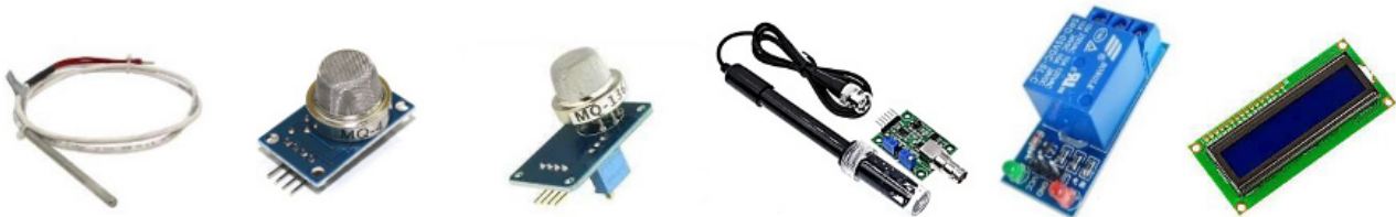
Figure 3. Shows the pH, gas, and temperature sensors as well as the relay module and LCD display.
