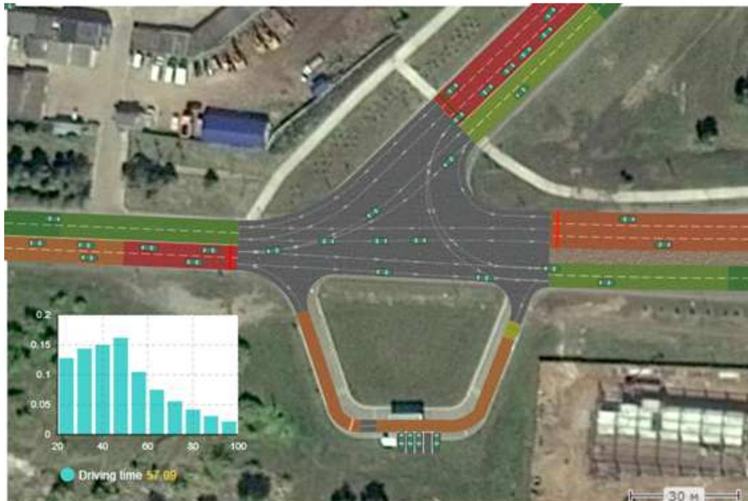
**Figure 2 – The results of the test of the intersection model with the current parameters of the traffic lights**
