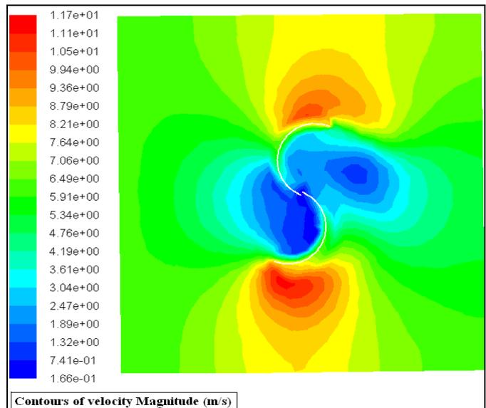
Fig. 6c. Velocity magnitude contour at  $90^\circ$  rotor.
