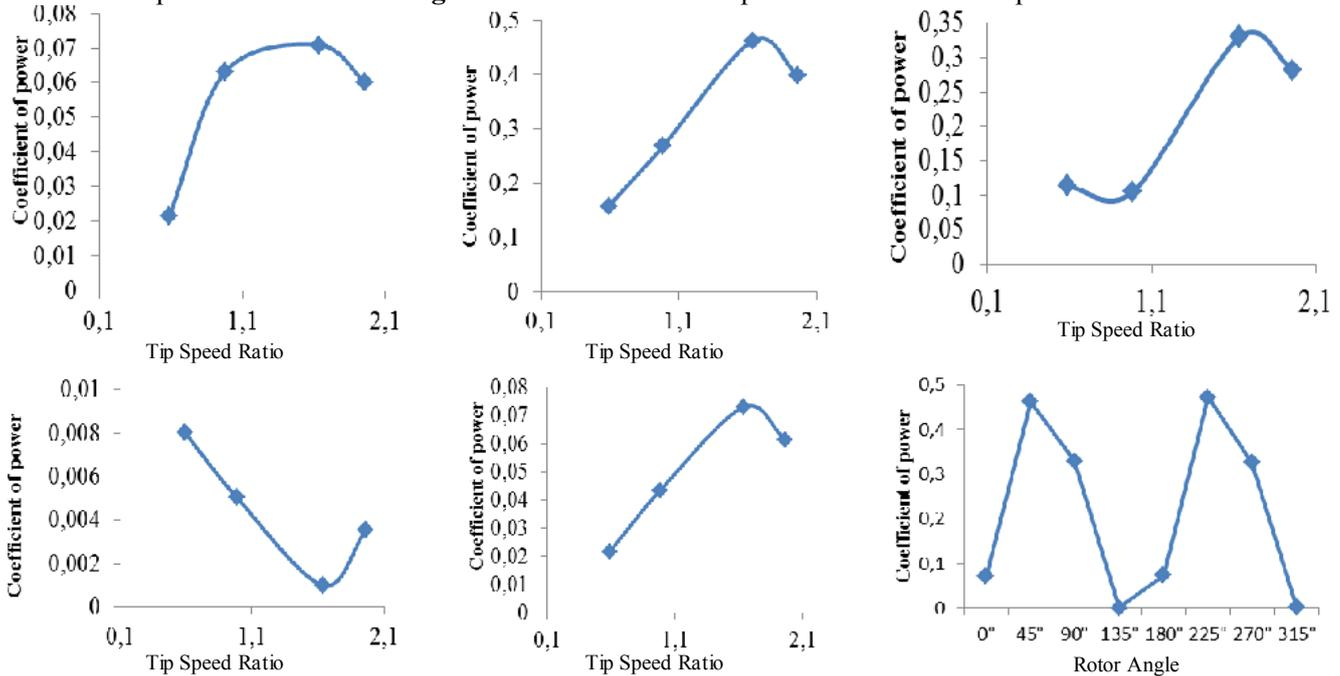
Fig. 3 (a) Variation of  $C_p$  at 0° rotor angle with TSR, (b) Variation of  $C_p$  at 45° rotor angle with TSR, (c) Variation of  $C_p$  at 90° rotor angle with TSR, (d) Variation of  $C_p$  at 135° rotor angle with TSR, (e) Variation of  $C_p$  at 180° rotor angle with TSR, and (f) Variation of  $C_p$  at complete cycle of rotation at maximum TSR=1.636.
