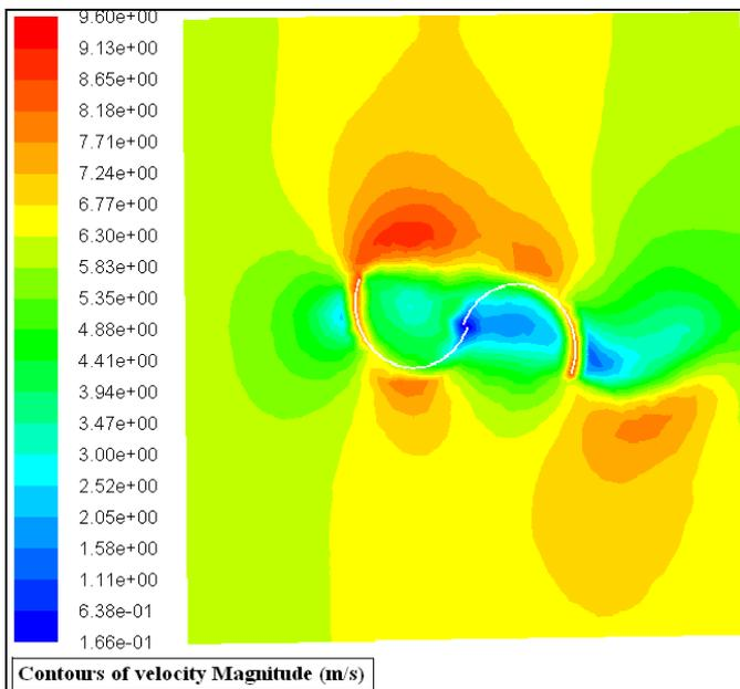
Fig. 6e. Velocity magnitude contour at 180° rotor.
