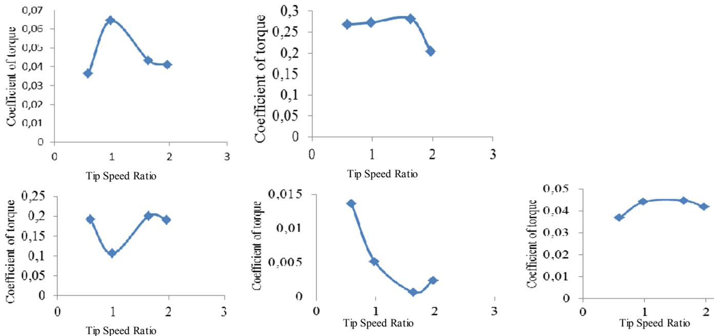
Fig. 4 (a) Variation of  $C_t$  at 0° rotor angle with TSR, (b) Variation of  $C_t$  at 45° rotor angle with TSR, (c) Variation of  $C_t$  at 90° rotor angle with TSR, (d) Variation of  $C_t$  at 135° rotor angle with TSR, and (e) Variation of  $C_t$  at 180° rotor angle with TSR.
