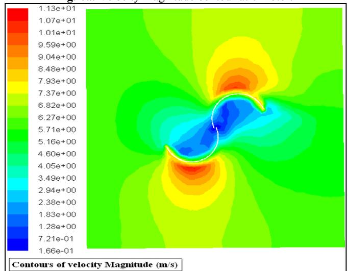
Fig. 6b. Velocity magnitude contour at  $45^\circ$  rotor.
