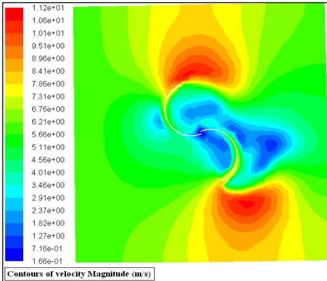
Fig. 6d. Velocity magnitude contour at 135° rotor.
