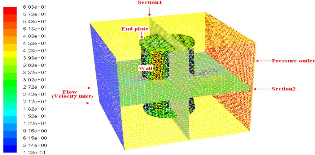
Fig. 2 Computation sections in the 3-D flow field.
