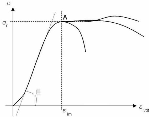
Fig. 5 Stress-strain curve – Strain measured by LVDT
