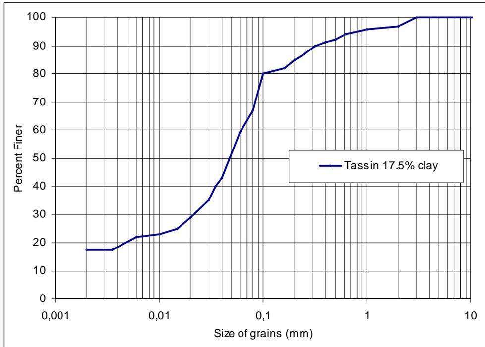
Fig. 1 Grading curve for T17.5% clay
