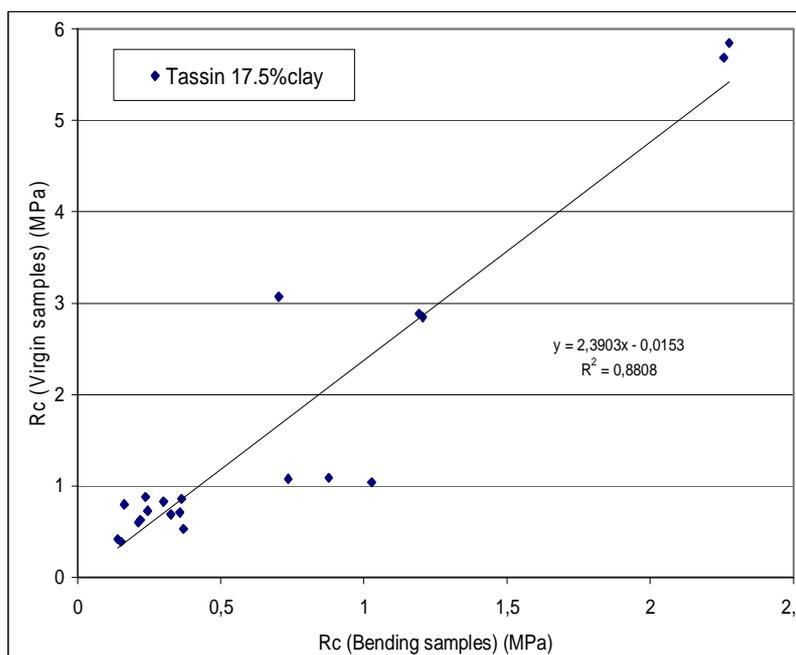
Fig. 7 Comparison between compressive strength belonging to virgin samples and others coming from bending tests – Tassin mortars (non stabilized and stabilized formulations).
