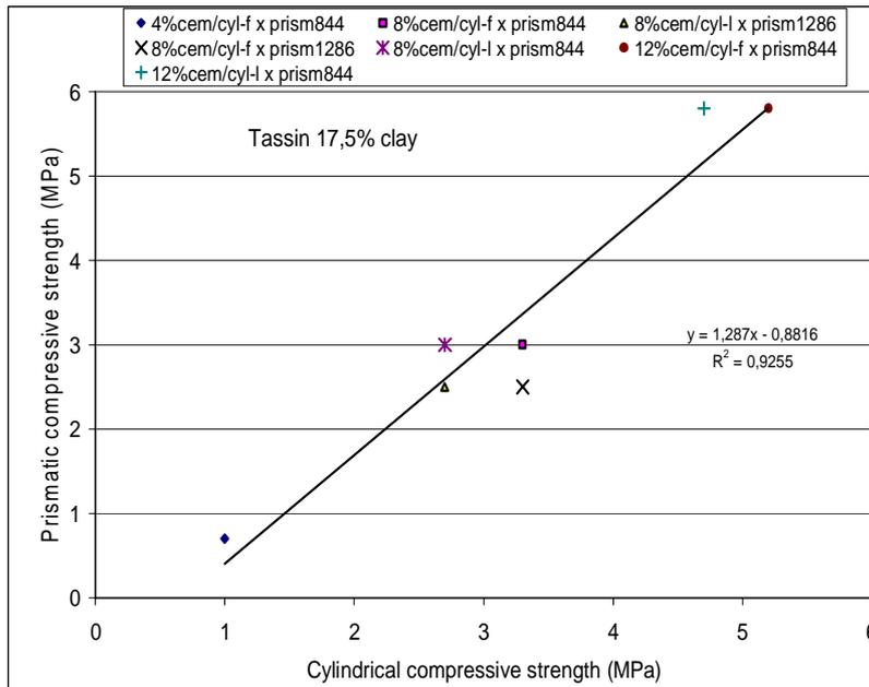
Fig. 6 Comparison between cylindrical and prismatic compressive strengths.
