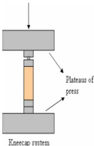
Fig. 3 Two types of experimental devices of kneecap
