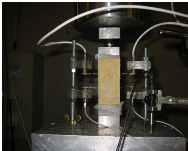
**Fig. 4** Experimental device adopted as optimum for simple compression test.
