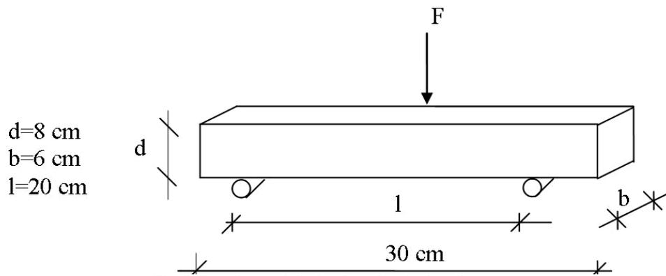
Fig. 2 Experimental device for a 3 point bending test.
