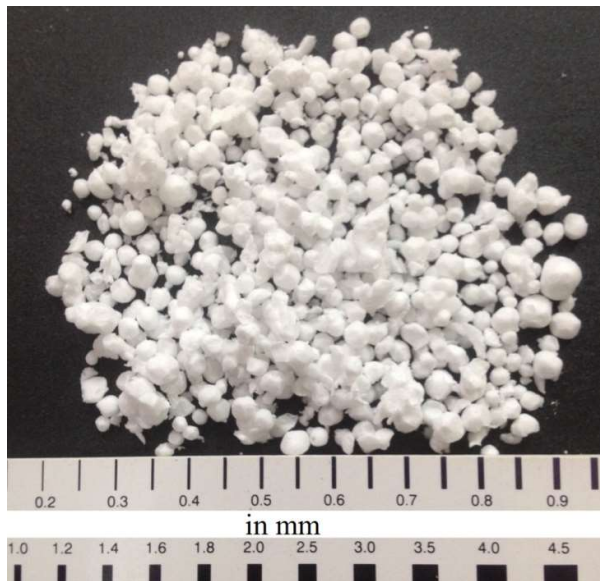
Fig. 2 Expanded polystyrene grains.
