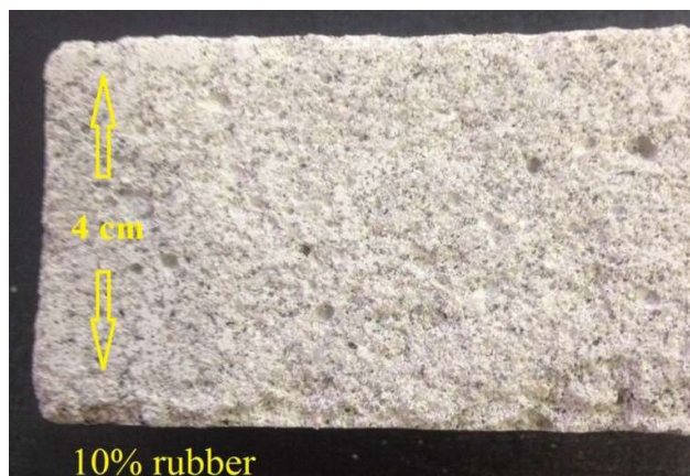
Fig. 9 Aspect of mortar with 10% of rubber.
