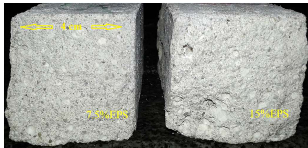
Fig. 8 Aspect of mortar with 7.5% and 15% of EPS.
