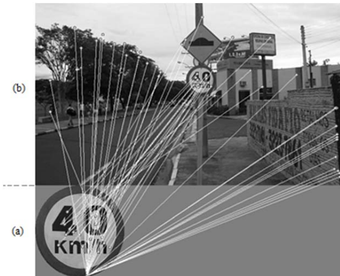
Fig. 2 Matching between a) template and b) input image, after the keypoints after evaluation of the 128 SIFT features.
