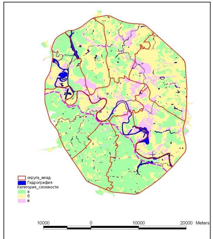
**Fig. 2.** Schematic map of engineering geological complexity (fragment of the city of Moscow territory inside Moscow Ring Road (MKAD) with boundary between uplift (A) and subsidence (B) megamassifs (dotted crimson line).
