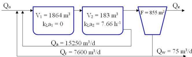
Fig. 10 The size of the WWTP for case B after optimization
