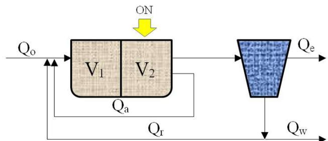
Fig. 5 Nitrogen reduction by aerobic and anoxic tanks
