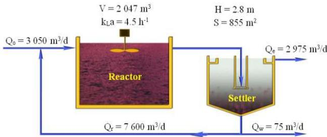
Fig. 1 Typical activated sludge treatment plant
