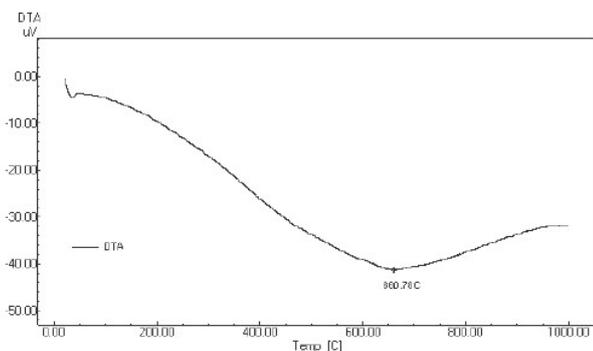
**Fig. 5** DTA curve from the differential thermal analysis of the slurry sample.
