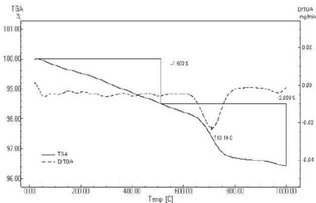
**Fig. 4** TG and drTG curves from thermogravimetric analysis of the slurry sample.
