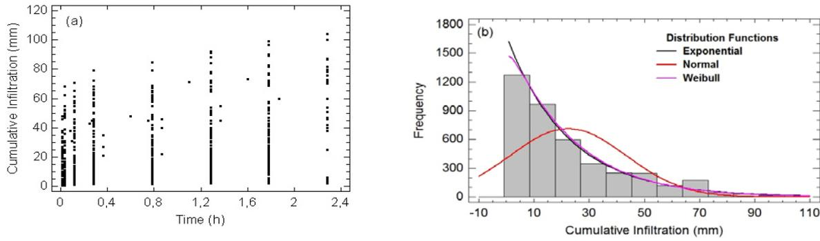
**Fig. 7** Cumulative infiltration depth: (a) temporal variation, and (b) frequency histogram and predicted Weibull probability density function.
