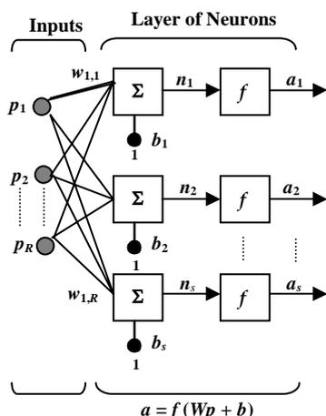
**Fig. 2** Single layer network architecture of neurons.
