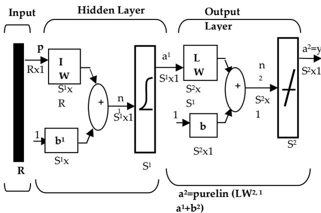
**Fig. 5** Architecture of a feedforward network.
