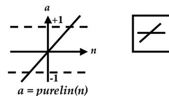
**Fig. 4** Lineal transfer function.
