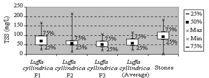
**Fig. 10** Box-whisker graphics for total suspended solids (TSS) downstream the filters filled with *Luffa cylindrica* (F1, F2, F3 and average value) and downstream the filter filled with stones (upstream the secondary settlers).
