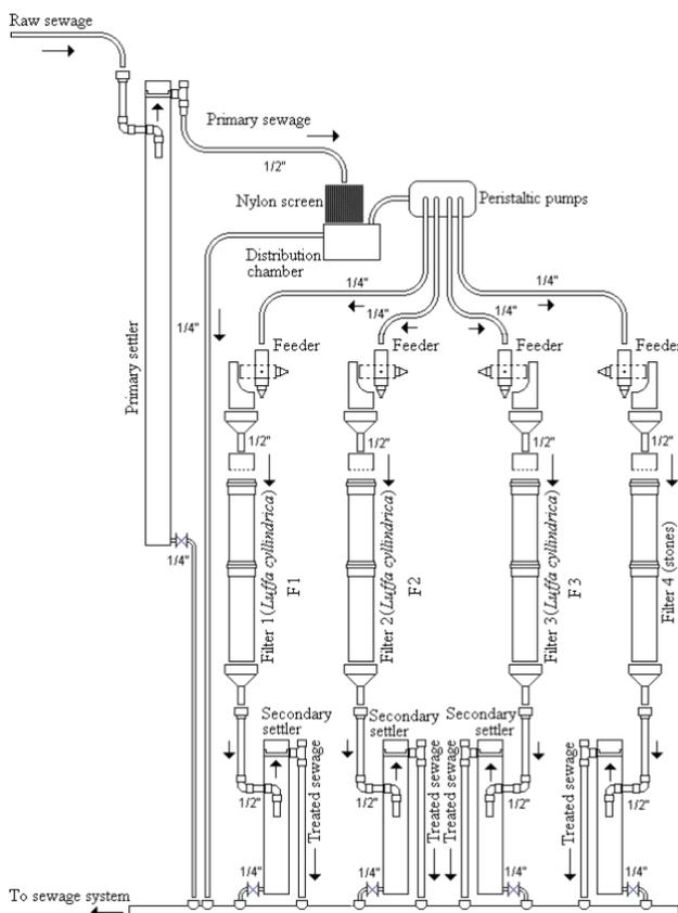
**Fig. 3** General arrangement of the pilot plant, consisting of a primary settler, and four parallel and identical secondary biologic systems, three of them operating with *Luffa cylindrica* as biofilm support medium (F1, F2, F3), and the last one using stones (filter 4).
