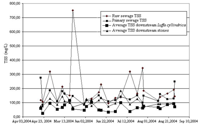
**Fig. 9** Total suspended solids (TSS) in raw and primary sewage, downstream the filters filled with *Luffa cylindrica* and downstream the filter filled with stones (upstream the secondary settlers): temporal series.
