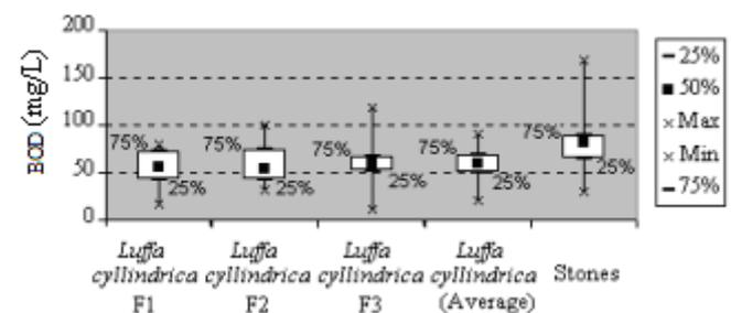
**Fig. 6** Box-whisker graphics for biochemical oxygen demand (BOD<sub>5,20</sub>) downstream the filters filled with *Luffa cylindrica* (F1, F2, F3 and average value) and downstream the filter filled with stones (upstream the secondary settlers).
