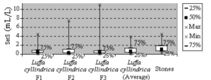
**Fig.12** Box-whisker graphics for settleable solids (SetS) downstream the filters filled with *Luffa cylindrica* (F1, F2, F3 and average value) and downstream the filter filled with stones (upstream the secondary settlers).
