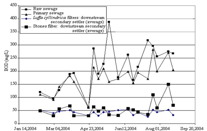
**Fig. 5** Biochemical oxygen demand (BOD<sub>5,20</sub>) in raw and primary sewage, downstream the trickling filters filled with *Luffa cylindrica* and downstream the filter filled with stones: temporal series.
