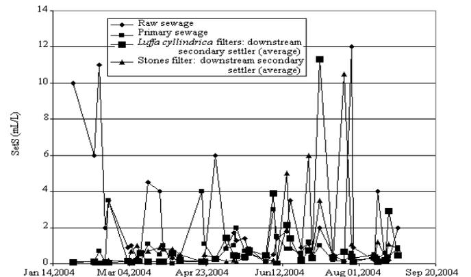
**Fig. 11** Settleable solids (SetS) in raw and primary sewage, downstream the trickling filters filled with *Luffa cylindrica* and downstream the filter filled with stones: temporal series.
