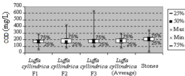
**Fig. 8** Box-whisker graphics for chemical oxygen demand (COD) downstream the filters filled with *Luffa cylindrica* (F1, F2, F3 and average value) and downstream the filter filled with stones (upstream the secondary settlers).
