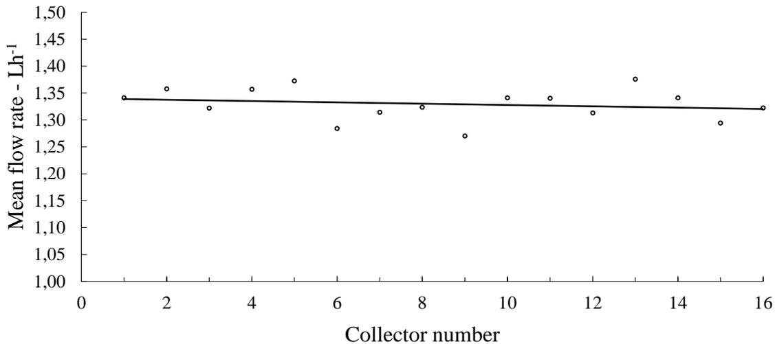
**Figure 5.** Distribution of the dripper flow rates in the evaluation of the system.
