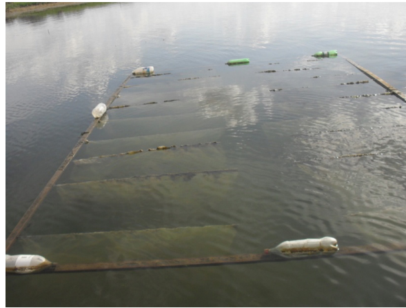
Figure 2 - Floating structures, using plastic for fixing the biofilme, applied at Taperoá Dam. Photo: Cristina Crispim 2013.
