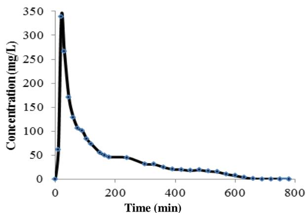
**Fig. 12** First cycle desorption profile of CV.
