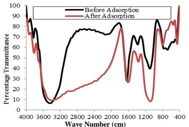
**Fig. 10** FTIR Spectrum of bottom ash before and after CV adsorption.
