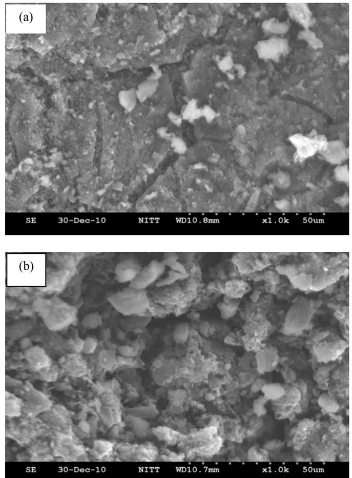
**Fig. 9** SEM micrographs of bottom ash: (a) before adsorption; (b) after adsorption.
