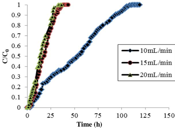
Fig. 6 Effect of flow rate on breakthrough curves.
