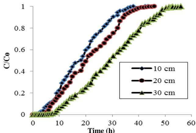
Fig. 4 Effect of bed depth on breakthrough curves.
