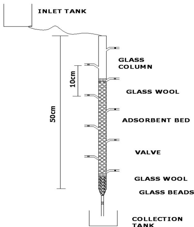
Fig. 2 Schematic diagram of lab-scale column study.
