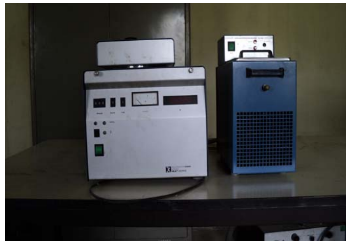
Fig. 3 Photograph of Bomb Calorimeter used in the study.
