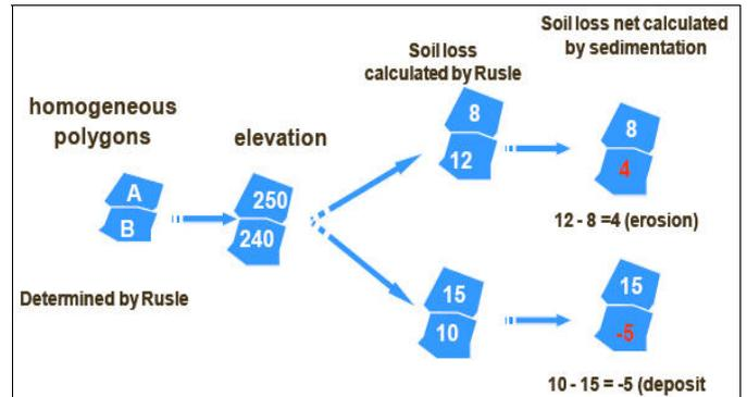
**Fig. 4** Principle model of deposition: Sedimentation (El Garouani, 2007).
