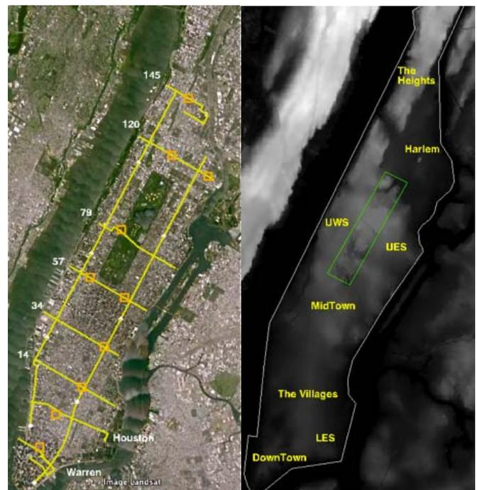
**Fig. 1** Mobile instrument pedestrian routes and fixed instrument locations (a, left). Elevations and neighborhoods (b, right).
