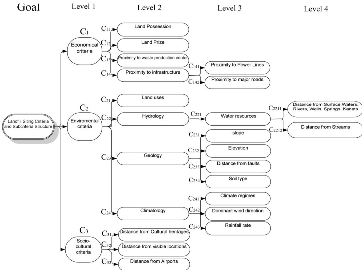
Fig. 7 Hierarchy structure of landfill sitting AHP model.
