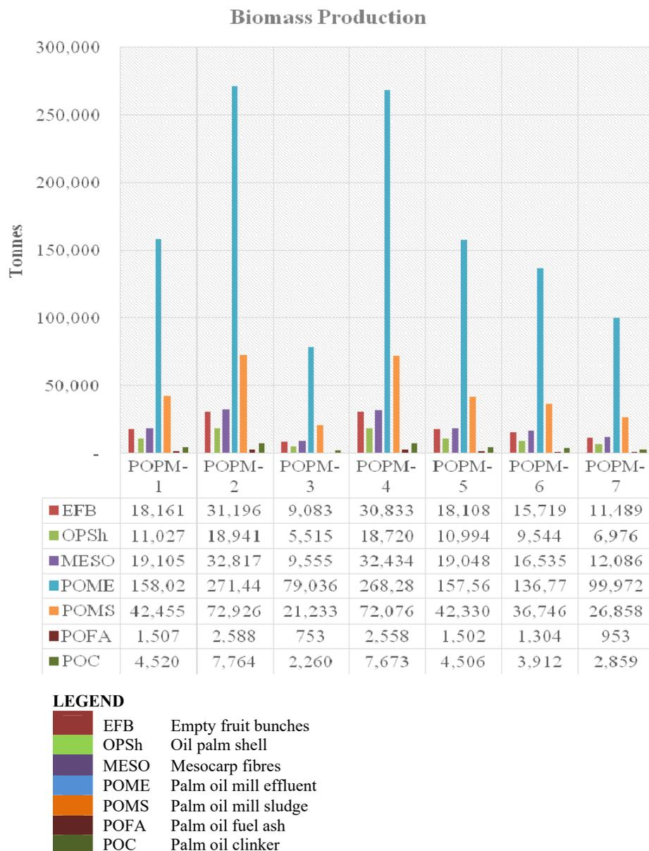
**Fig.1** An approximation of the oil palm processing wastes generated per annum in the inspected palm oil mills
