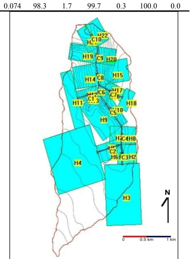
Fig. 4 Discretization of Guaraira river experimental basin for the WEPP model.
