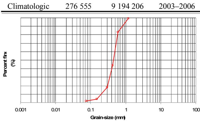
Fig. 2 Grain-size distribution curve for the bed material.
