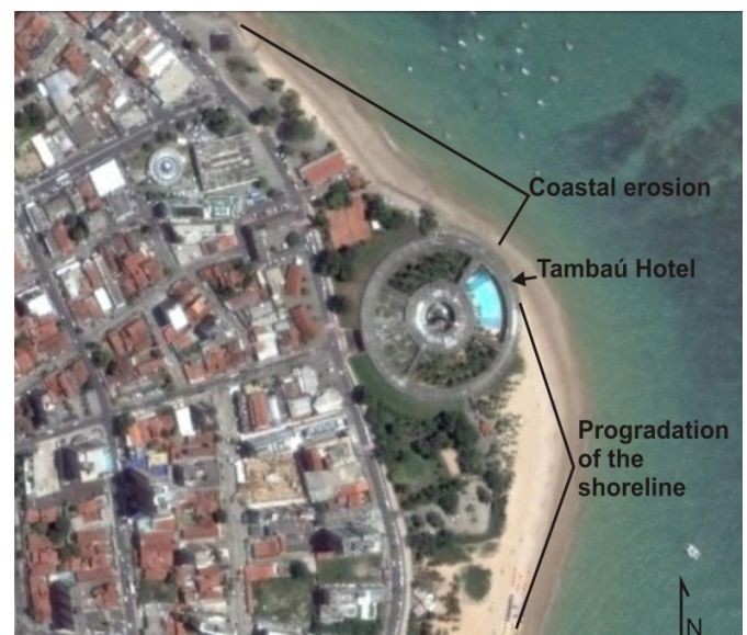
Fig. 6 Hotel Tambaú showing the prograding Tambaú Beach to the south and the eroding Manaíra Beach to the north.
