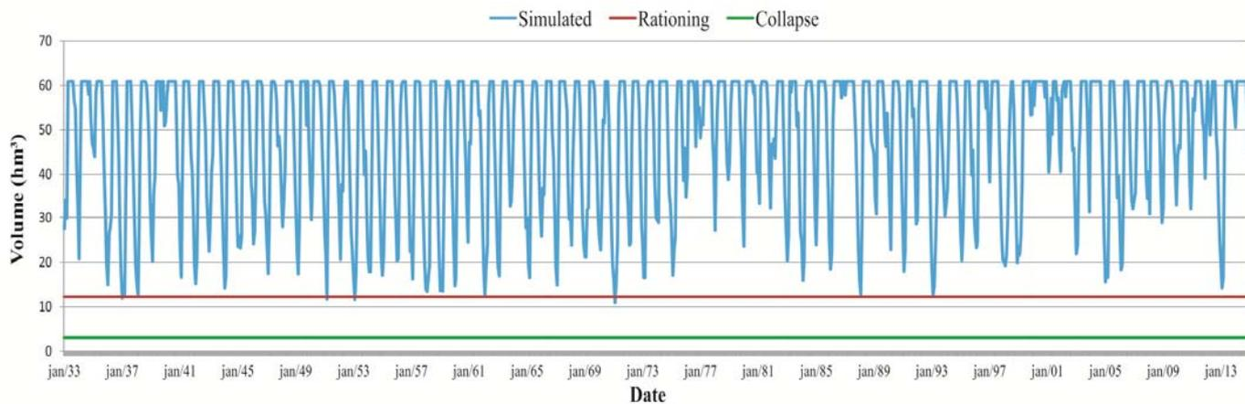
Fig. 9 Simulated storage considering the alternative operation rules for Pirapama reservoir.
