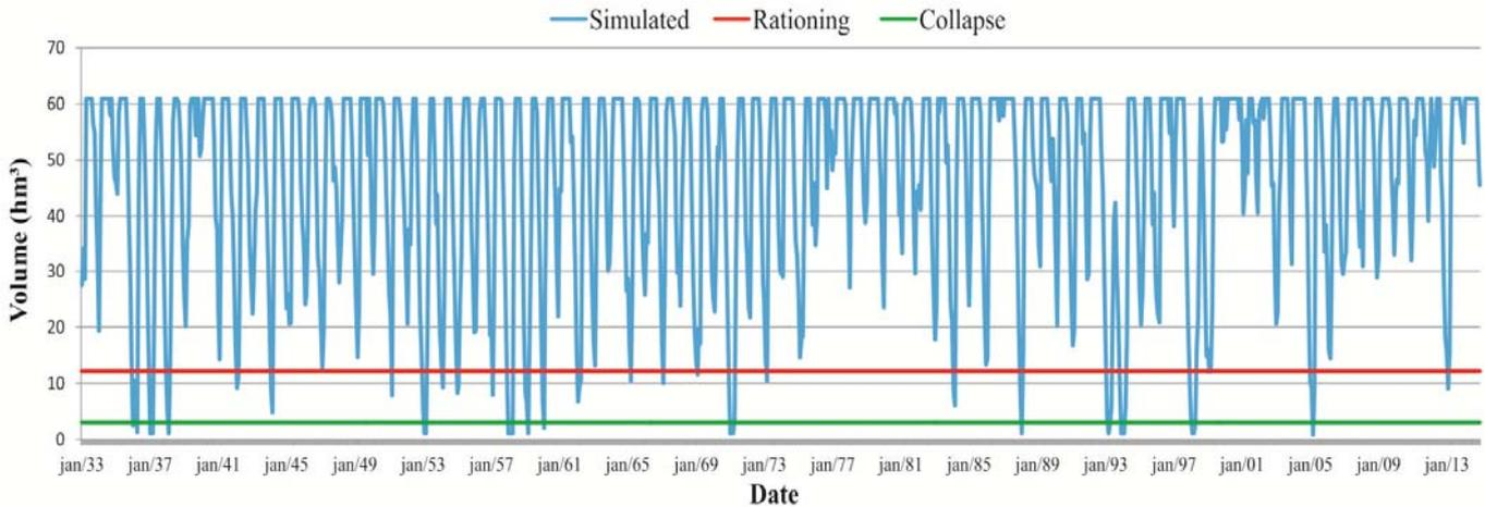
Fig. 8 Simulated storage considering the current operation rules.
