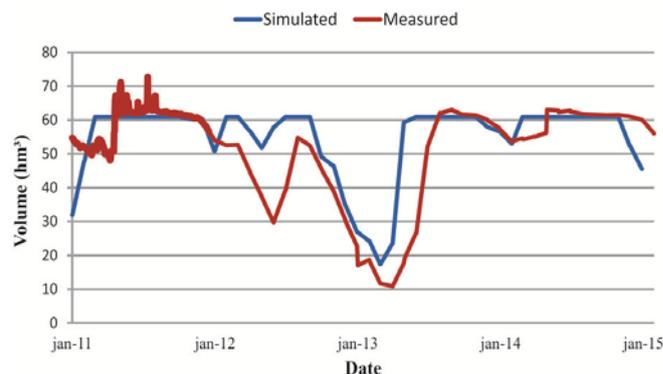
**Fig. 7** Measured and simulated storage in the Pirapama reservoir.**Table 6.** Amount of months per reservoir condition.
