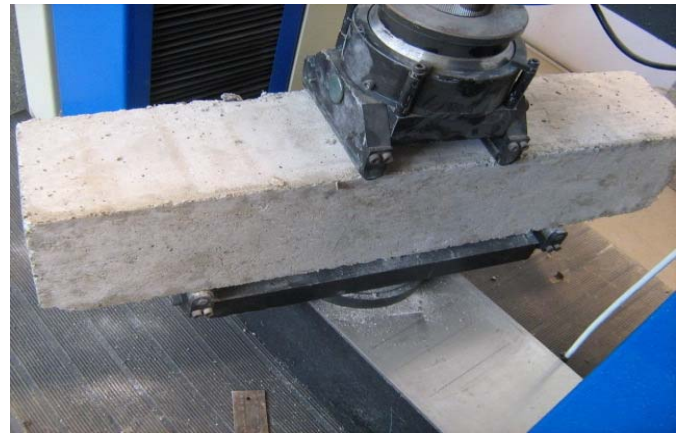
Fig. 2 Flexural strength test.
