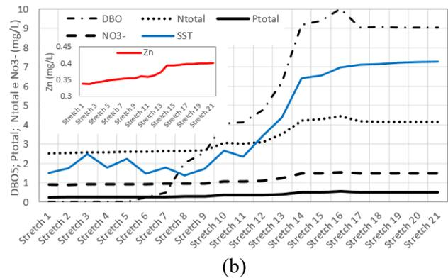
**Fig. 4** (a) Identification of stretches 9 and 16 of Lageado Stream; (b) Longitudinal distribution of the concentrations of pollutants in Lageado Stream for the 30-year urbanization scenario.
