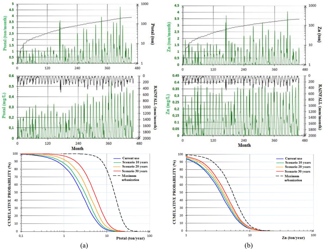
Fig. 7 Probable series of loads and concentrations in the Lageado Basin, considering a horizon of 38 years, where: (a)  $P_{total}$  and (b) Zinc.
