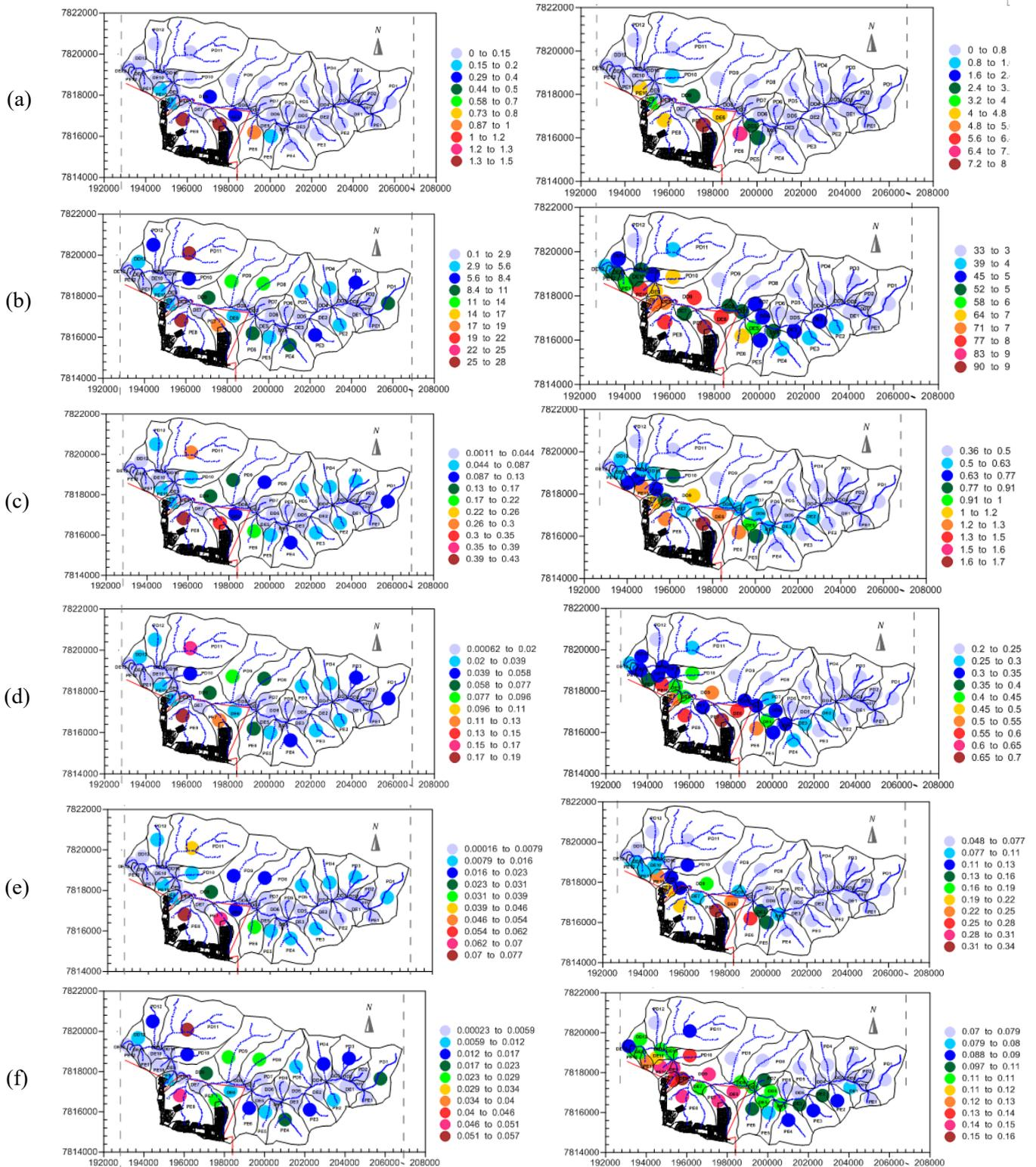
**Fig. 3** Spatial distributions, for a 10-year urbanization scenario, of the probable mean loads and concentrations generated in each sub-basin contributing to Lageado Stream for the parameters: (a) BOD, (b) TSS, (c)  $N_{total}$ , (d)  $NO_2^-$  and  $NO_3^-$ , (e)  $P_{total}$  and (f) zinc.
