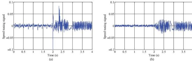
**Fig. 11** Open loop estimation 20 r/min and 75% load, speed tuning signal. (a) Classical MRAS. (b) Predictive MRAS. estimator at all operating speeds
