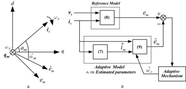
Fig 3 Back-EMF error-based MRAS: (a) Coordinates in stationary reference frame, (b) Structure of back-EMF error-based MRAS system for speed estimation (Saejia & Sangwongwanich, 2006)
