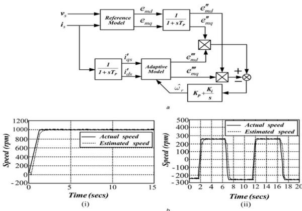
**Fig 4** Back-EMF error-based MRAS (a) Speed estimator ,(b) Performance of a back-EMF-based MRAS speed estimator for  $\hat{v}_r$  :
