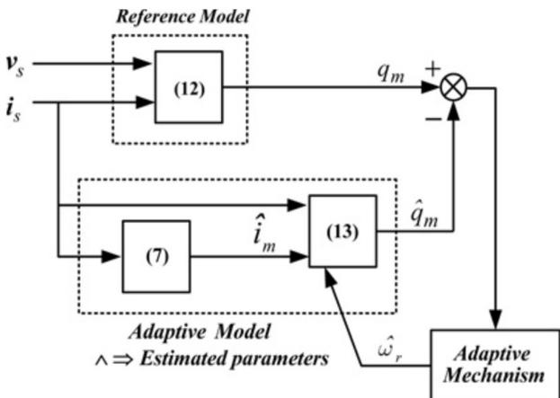
Fig 5 Basic structure of reactive power-error-based MRAS system for speed estimation (Saejia & Sangwongwanich, 2006) are achieved.
