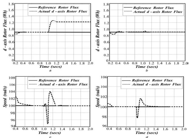
**Fig.1** Simulation results for rotor-flux-error-based MRAS (Shen *et al.*, 2014): actual and reference rotor fluxes, (a) Without rotor resistance estimator, (b) With rotor resistance estimator, actual and reference rotor speed, (c) Without rotor resistance estimator, (d) With rotor resistance estimator.
