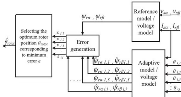
Fig.7 Block diagram of the proposed MRAS estimator.
