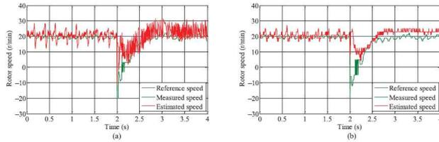
**Fig. 10** Open loop estimation, 20 r/min and 75% load, rotor speed. (a) Classical MRAS. (b) Predictive MRAS.
