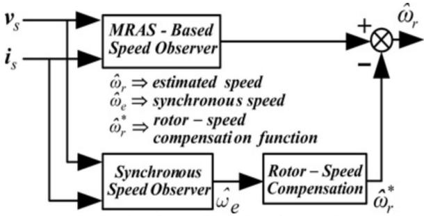
Fig. 2 MRAS-based rotor-flux-oriented speed observer scheme (Suwankawin & Sangwongwanich, 2006)
