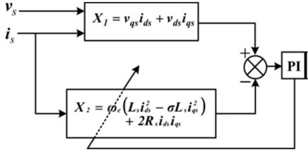
Fig. 6 X-MRAS structure for rotor speed estimation NEW X-MRAS
