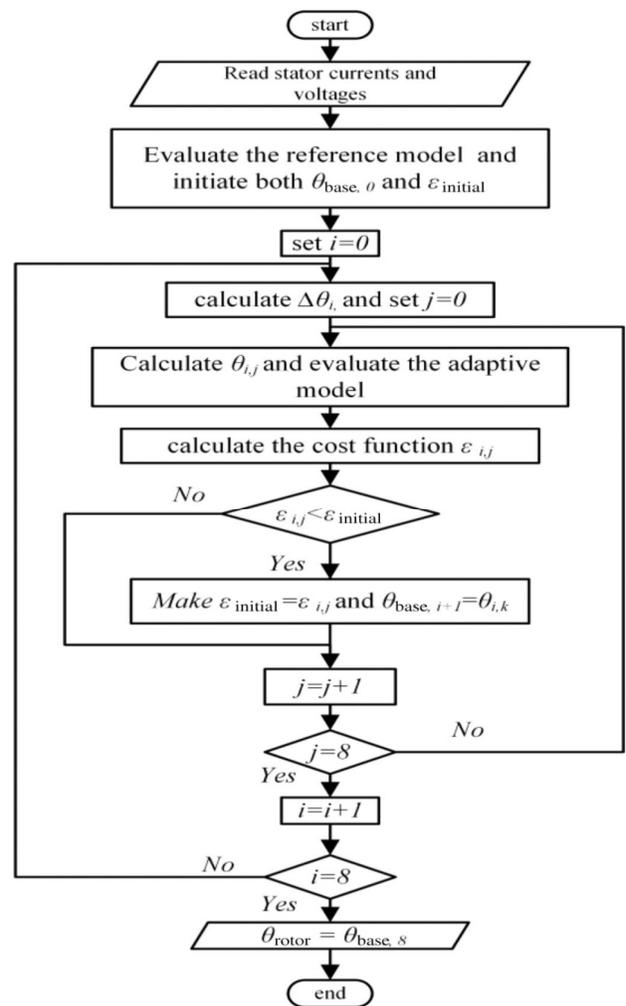
Fig. 9 Flowchart of the rotor position search algorithm.
