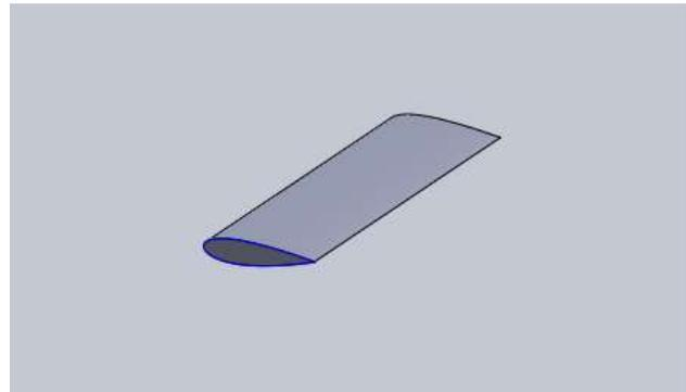
**Fig. 8** Extrude airfoil
