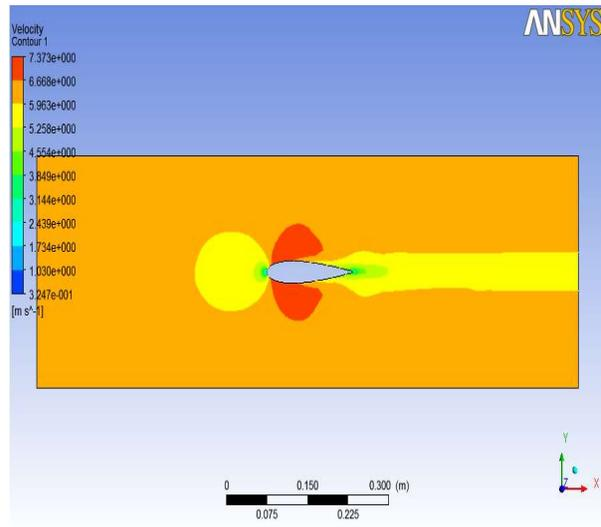
Fig. 11 velocity contours for 6 m/s wind velocity
