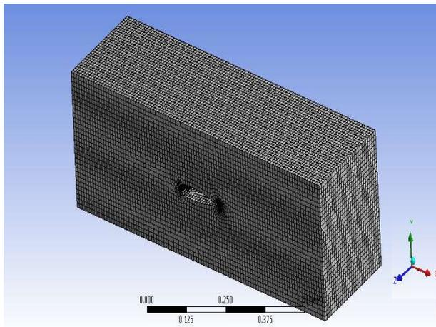
Fig. 10 Meshing of NACA 0018 airfoil
