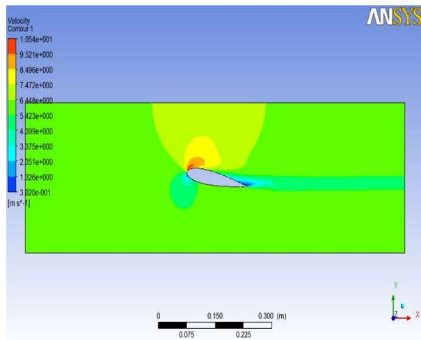
Fig. 12 velocity contours for 6 m/s wind velocity
