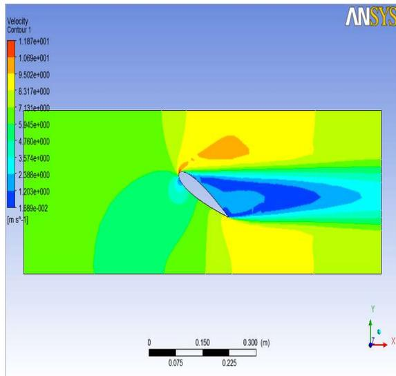
Fig. 14 velocity contour for 6 m/s wind velocity.
