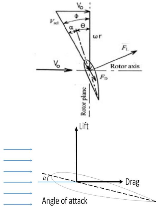
Fig. 2 Velocity and force diagram.
