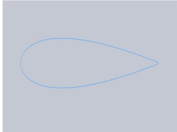
**Fig. 7** NACA 0018 Airfoil in solid works
