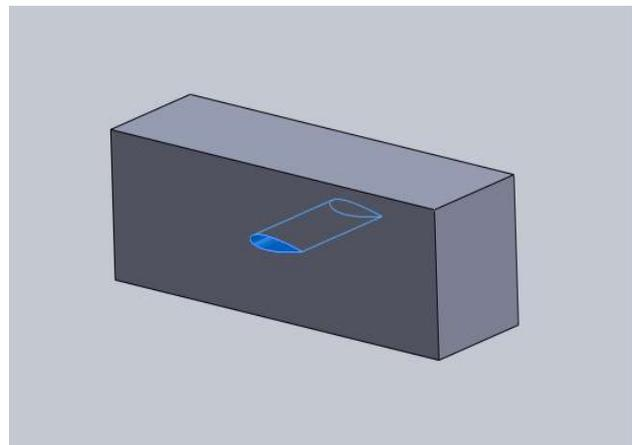
**Fig. 9** Create cavity domain of above extruded airfoil.
