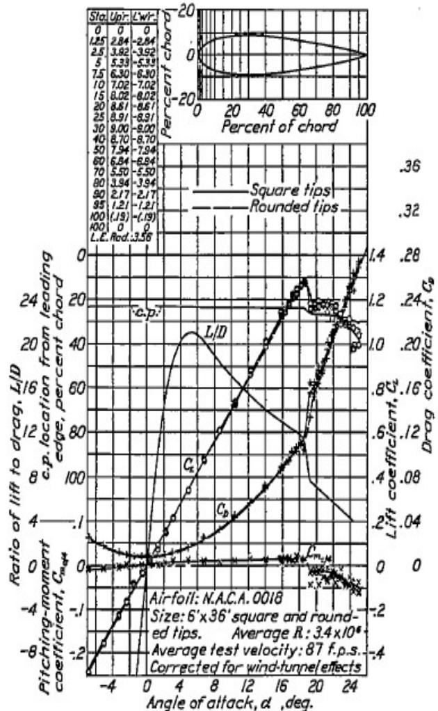
**Fig. 6** Characteristics of NACA 0018 airfoil
