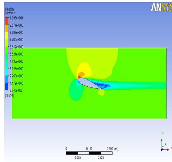
Fig. 13 velocity contours for 6 m/s wind velocity.
