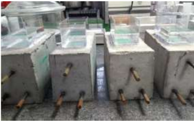
Fig. 3 Chloride ion induction acceleration method in concrete.
