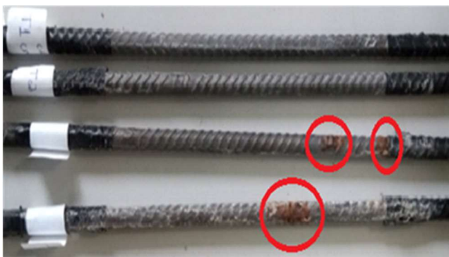
Fig. 7 Indication of signs of corrosion on steel specimens.
