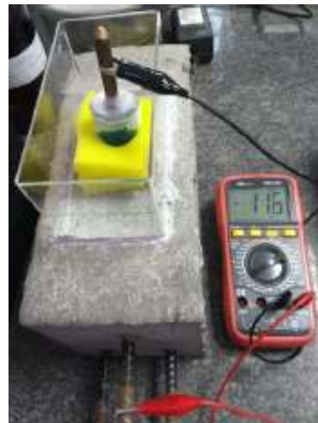
Fig. 4 Electrode potential measurement system using a voltmeter.
